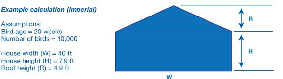
Design air speed (feet per minute or ft/min) = 400 ft/min (rearing) and 500 ft/min (production) Fan capacity at 0.15 inches of water column (ft<sup>3</sup>/min) = 20,585 ft<sup>3</sup>/min Cross section area =  $(0.5 \times W \times R) + (W \times H)$
